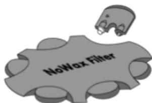
Push the removal arm of the tool into the existing NoWax filter in the RU as shown in illustration 1. Remove the used filter by pulling the tool away from the RU as displayed in illustration 2.
